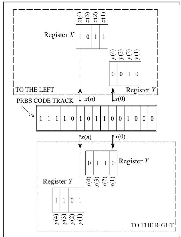
Figure 3. Error detection with two code reading heads
