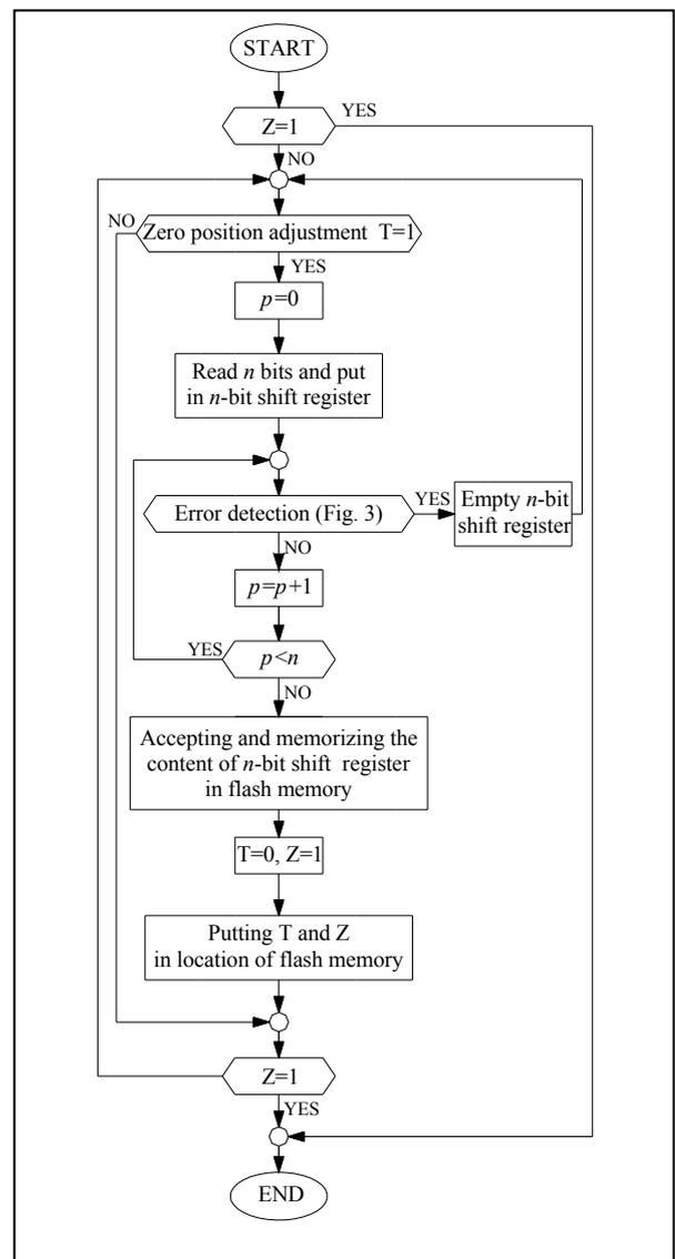
Figure 4. Direct zero position determination method
