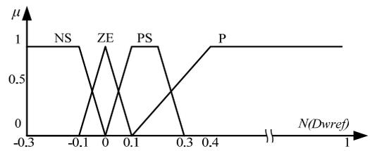
Fig. 6 Membership functions for input variable  $N(DWref)$
