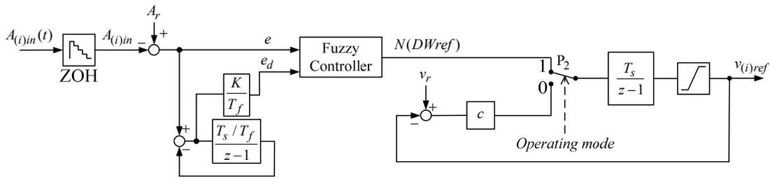
Fig. 3 Algorithm for generating the reference speed of the  $i$ -th BC in the BC system with FLC - case A
