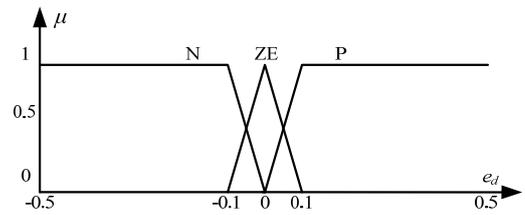
Fig. 5 Membership functions for input variable  $e_d$
