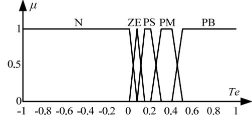
Fig. 11 Membership functions for input variable  $T_e$
