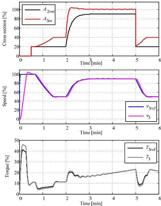
Fig. 7 Characteristic values of the third belt with FLC - case A: transition period from constant speed operation to controlled speed operation with changes of the incoming material from 20% to 90% of rated value and vice versa, in a realistic way that can be expected in practice
