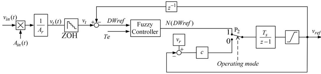
Fig. 9 Algorithm for generating the reference speed of the belt with FLC - case B
