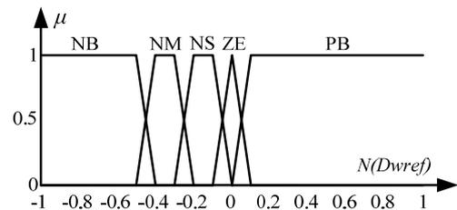
Fig. 12. Membership functions for output variable  $N(DWref)$ .
