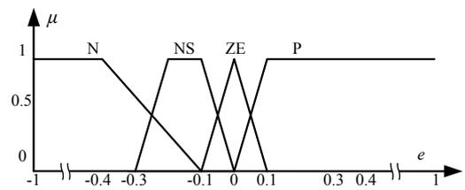
Fig. 4 Membership functions for input variable  $e$
