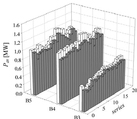
Fig. 15 Average power consumption of belt drives in [MW], on the third, fourth and fifth BC station (B3, B4 and B5): white bars - constant speed operation, grey bars - variable speed operation with FLC - case B
