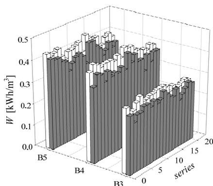
Fig. 16 Consumption of Energy per m<sup>3</sup> [kWh/m<sup>3</sup>], on the third, fourth and fifth BC station (B3, B4 and B5): white bars - constant speed operation, grey bars - variable speed operation with FLC - case B
