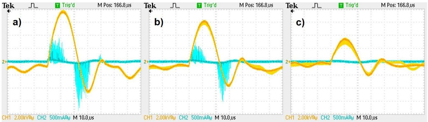
Figure 4. Current microdischarges through plasma actuator #1 operating at 10 kHz with applied voltage amplitudes of: a) 8 kV, b) 6 kV, c) 3 kV
