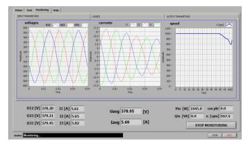
Figure 4. Screen display of INPUT PARAMETERS
