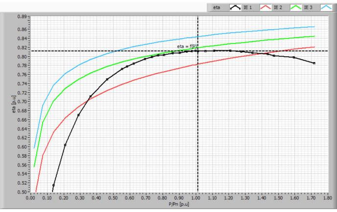
Figure 7. The motor efficiency compared to the curves of energy efficiency class boundaries
